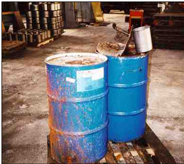
Hazardous waste illegally stored in open containers.
