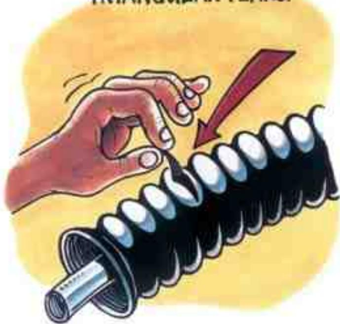
Sometimes customers catch the boot fabric on a sharp object near the gas cap. When this happens, the boot fabric can tear, usually in the shape of a triangle. Any tear longer than 1/2 inch on one side of the triangle is a defect and the boot must be replaced or repaired.
