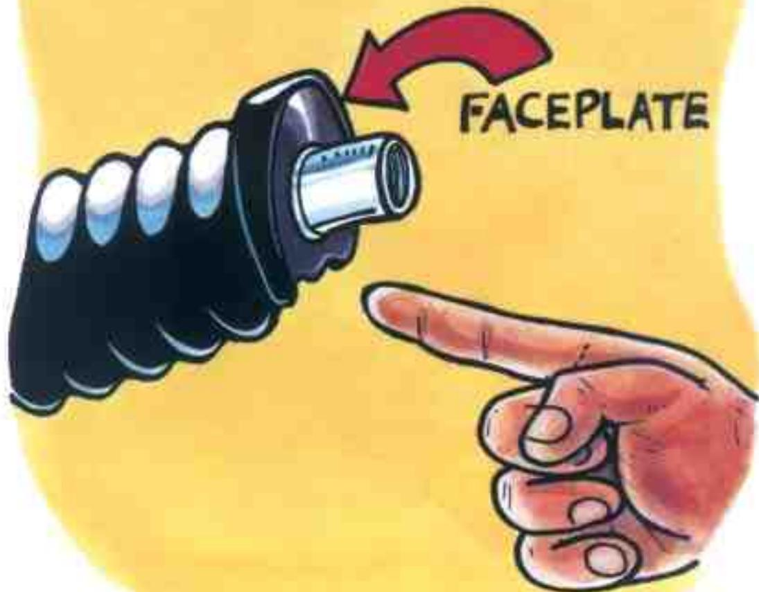
If your vapor recovery system nozzles have faceplates (balance system), replace any damaged or warped faceplates. The law requires that at least 3/4 of the faceplate circumference must make a good seal when used to dispense gasoline. Examine each nozzle faceplate daily to ensure that a good seal will occur and that at least 3/4 of the faceplate is intact. Again, it's best to replace any faceplate which does not provide a good seal with the automobile gas tank.
