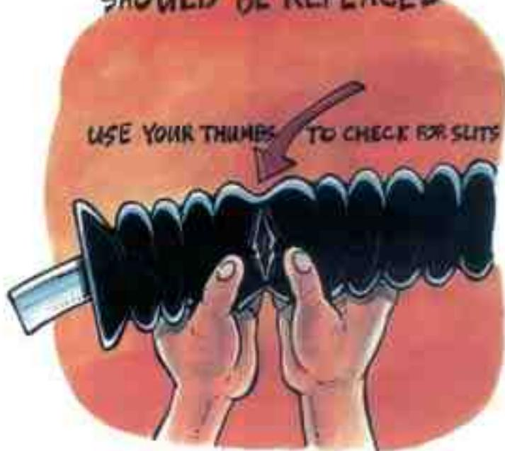
Wear and tear may cause slits to form in the folds of the boot fabric, which will cause a vapor leak. Use your thumbs to separate the ribs of the boot to check for these slits. Replace or repair all boots that have a slit one inch or longer. It's a good practice to replace any torn boot. **You cannot repair hoses or bellows with tape or duct tape.**
